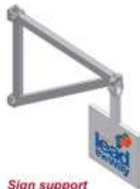
Sign support truss based on a right triangle
